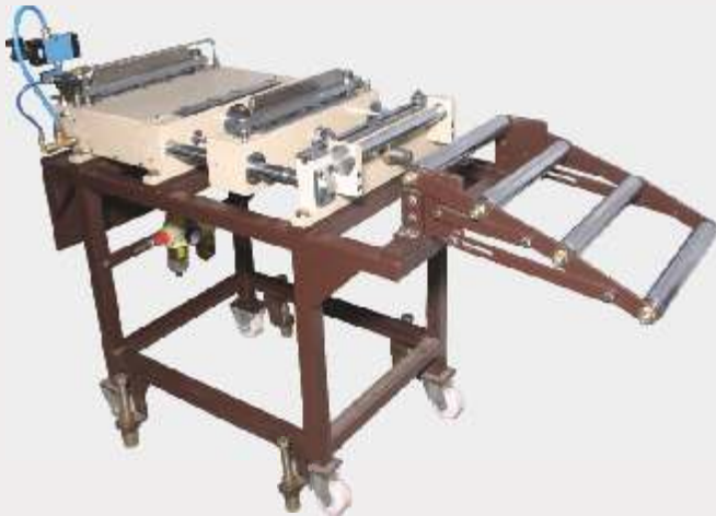
Extra Heavy Series Feeder Along with Cascade Rolls & Trolley type height adjustable mounting stand.
