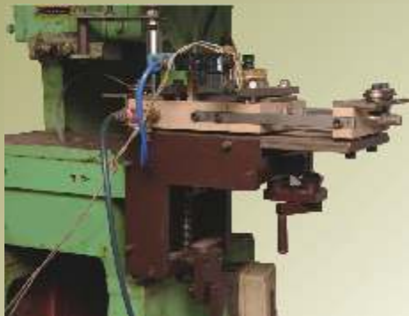
Feeder with universal mounting stand with x-y movement to clamp feeder on press & progressive tooling.
