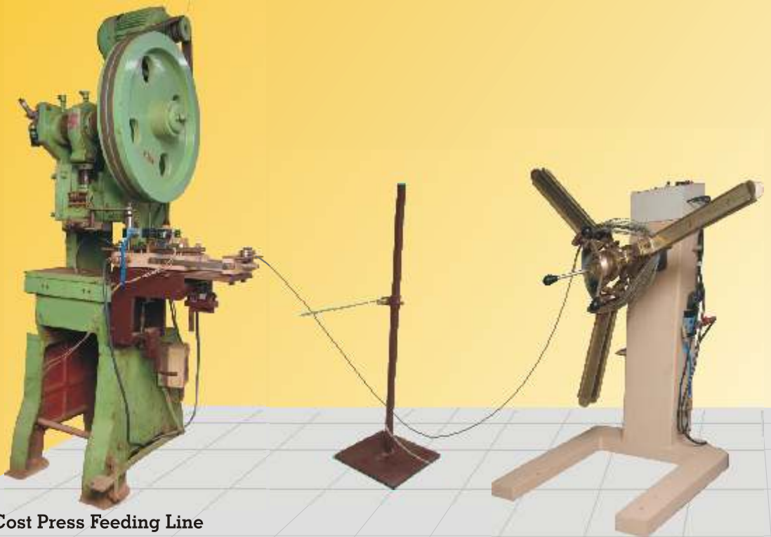
Extra Heavy Series Feeder Along with Cascade Rolls & Trolley type height adjustable mounting stand.
